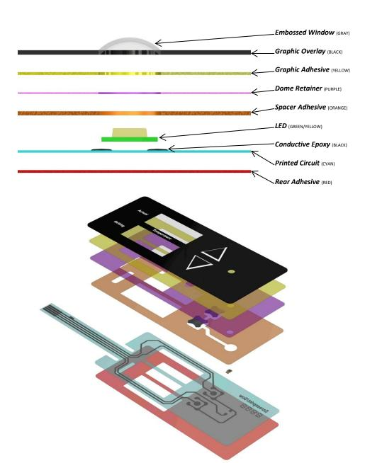
Design variations may include polyester dome, metal dome, or flat micro-motion membrane switches. The overlay may be flat or embossed, depending on design. Further integration is achieved by including printed Polymer Thick Film (PTF) resistors.
